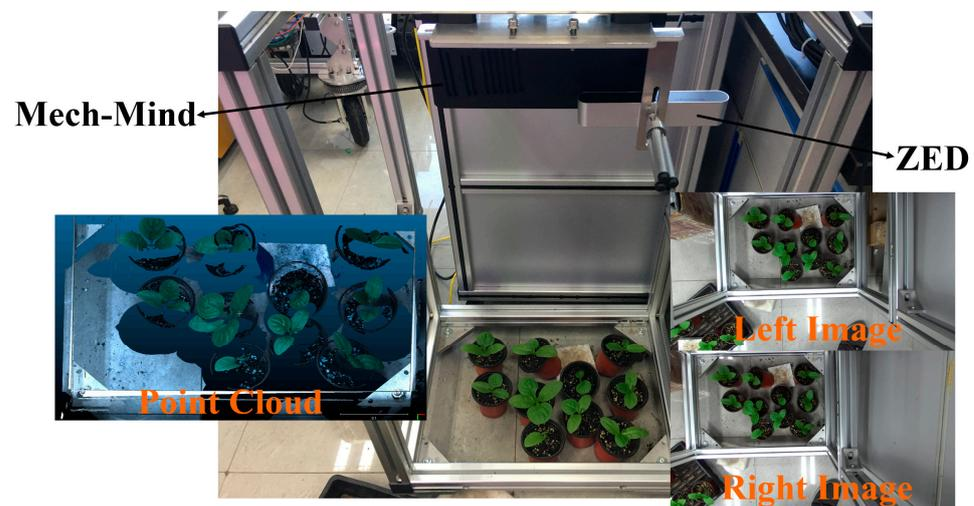
**Figure 1.** Data sampling system set up in this research. The system consists mainly of two cameras: binocular stereo ZED camera to obtain left and right view images for input and Mech-Mind Pro S Enhanced depth camera based on structured light to obtain depth information and generate disparity images for ground truth.
