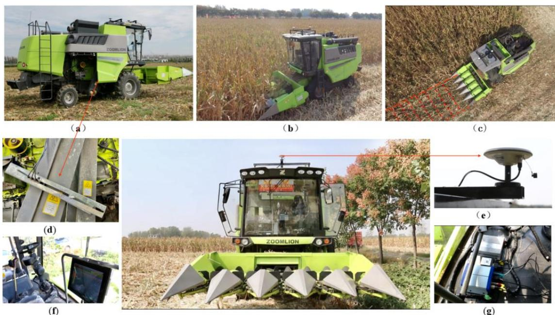
**Figure 6.** Field test scenes: (a) elevator position; (b) harvest scenes from field tests; (c) yield grids; (d) mounting position of the sensor; (e) BeiDou signal receiver; (f) display mounting position; (g) data processing side.
