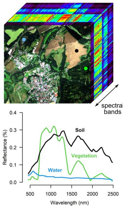
**Figure 6.** Data acquisition—an example of a CASI/SASI hyperspectral cube.
