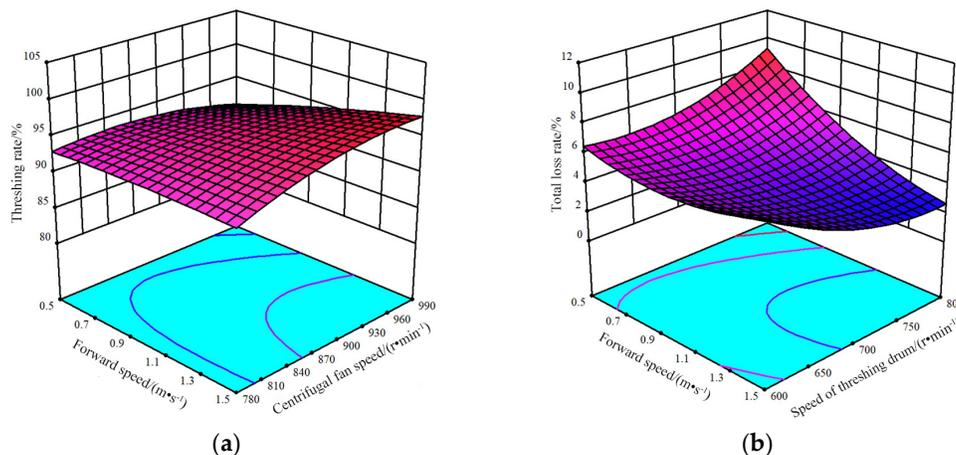
**Figure 13.** Influence of interaction factors on response values: (a) Effect of advancing speed and centrifugal fan speed on decontamination rate. (b) Effect of advancing speed and threshing drum speed on total loss rate.
