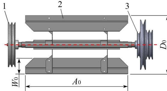
**Figure 10.** Schematic diagrams of the centrifugal fan structure: (1) Centrifugal fan power input pulley. (2) Fan blade. (3) Centrifugal fan power output pulley. Note:  $D_0$  is the diameter of the centrifugal fan in mm;  $A_0$  is the width of the centrifugal fan blade in mm;  $W_0$  is the height of the centrifugal fan blade in mm.
