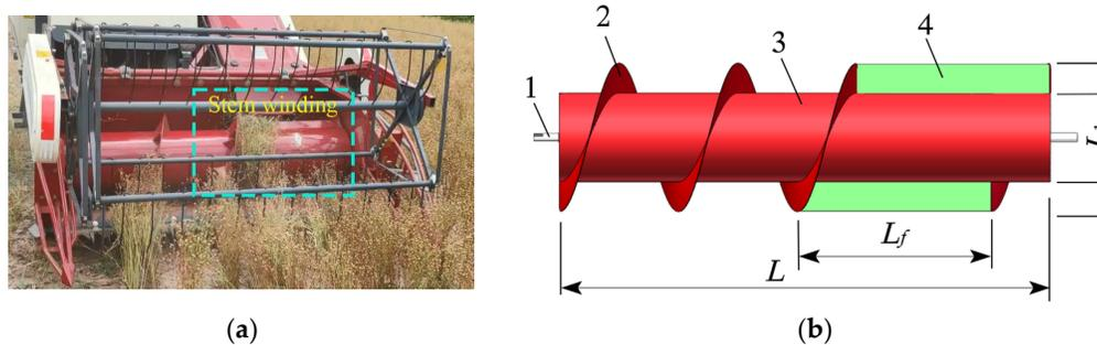
**Figure 3.** Diagram of the churn winding and anti-winding device: (a) Churning dragon wrap. (b) Diagram of the anti-tangle device. (1) Churning dragon wrap. (2) Diagram of the anti-tangle device. (3) Stirrer. (4) Anti-winding plate. Note:  $L$  is the length of the churn in mm.  $L_f$  is the length of the anti-winding plate in mm.  $L_1$  is the diameter of the churn in mm.  $L_2$  is the long shaft of the anti-winding churn in mm.
