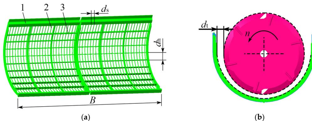
**Figure 7.** Schematic diagram of the structure of the narrow grid recess: (a) Concave plate size. (b) Concave plate-clad corners. (1) Narrow grating concave sieve. (2) Grating bars. (3) Horizontal spacer. Note:  $d_s$  is the spacing between the grating bars in mm;  $d_h$  is the spacing between the horizontal dividers in mm;  $d_t$  is the gap between the concave plates in mm.
