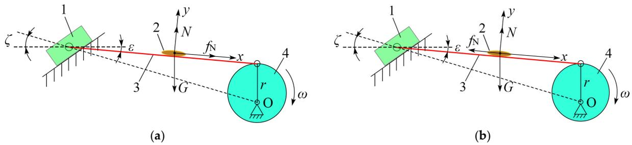
**Figure 9.** Kinematic model of a vibrating screen: (a) Slip-on detachment. (b) Slippage of debris. (1) limit slider. (2) Flaxseed grain. (3) Sieve surface. (4) Eccentric wheel. Note:  $G$  is the gravity of the flaxseed grain,  $N$ ;  $N$  is the support force on the flaxseed grain,  $N$ ;  $fN$  is the friction force on the sieve surface on the flaxseed grain,  $N$ ;  $\omega$  is the angular speed of the eccentric bearing in  $\text{rad}\cdot\text{s}^{-1}$ .
