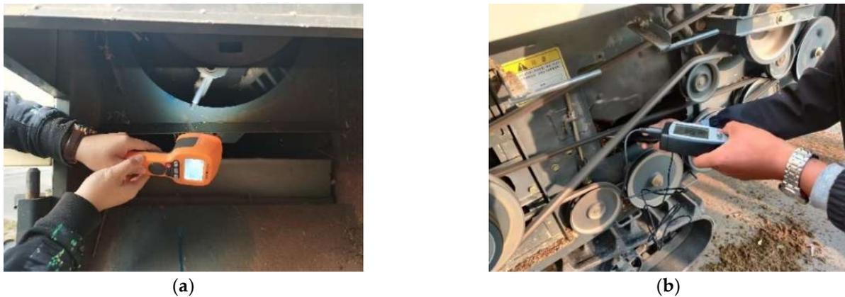
**Figure 11.** Determination of threshing drum speed and centrifugal fan airspeed on the prototype: (a) Threshing drum speed determination. (b) Centrifugal fan outlet air velocity determination.
