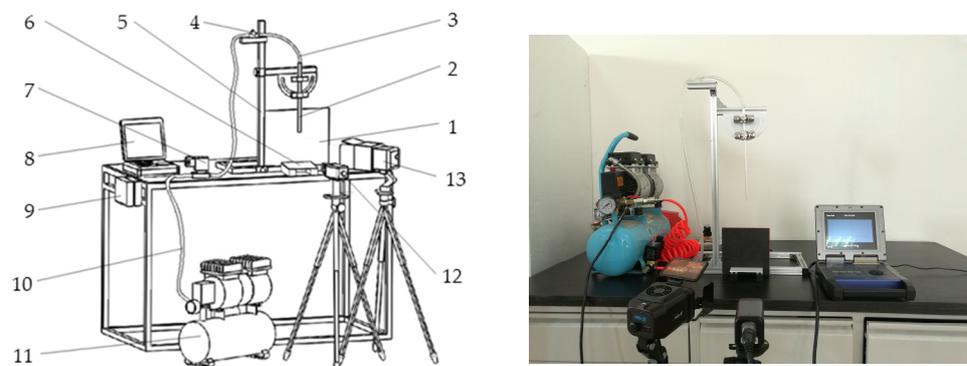
**Figure 3.** Image capture and testing system for fertilizer particle state during impact process: 1. back-board; 2. jetting tube; 3. guide tube; 4. feeding tube 5. support 6. target board; 7. solenoid; 8. analyzer host; 9. controller; 10. air pipe; 11. air compressor; 12. high speed camera; 13. light source.
