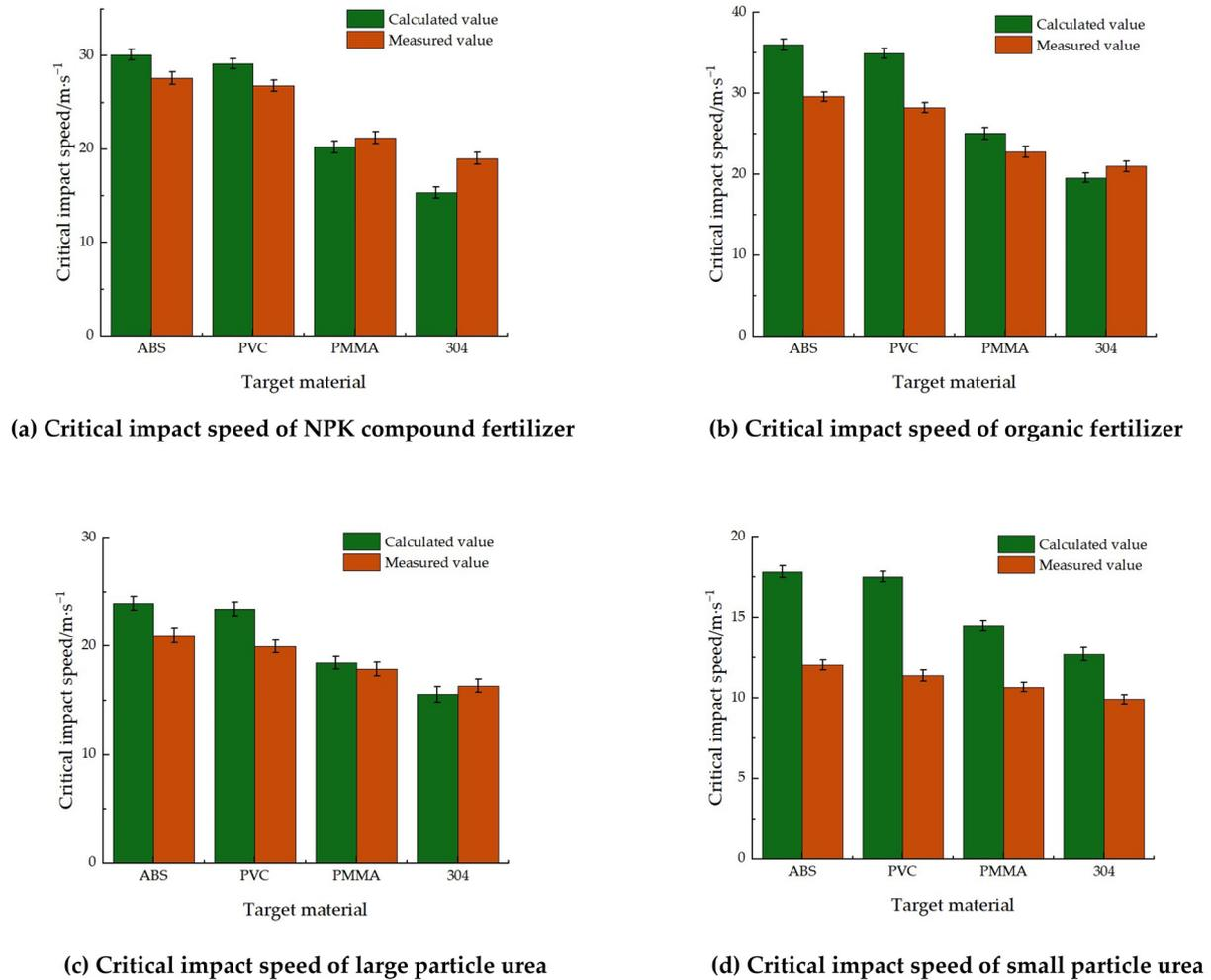
**Figure 8.** Comparison between calculated value and measured value of critical impact speed of fertilizer particles.
