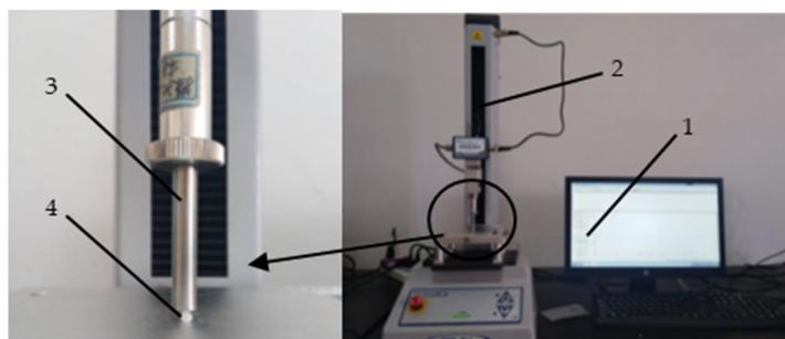
**Figure 4.** Fertilizer particle compression test: 1. computer; 2. texture analyzer; 3. indenter; 4. fertilizer particle.
