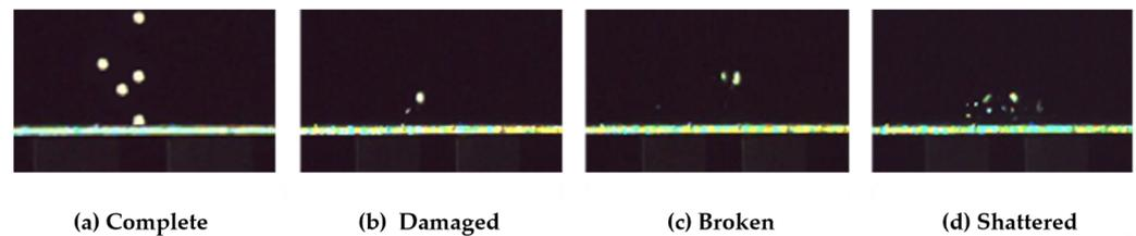
**Figure 5.** Typical states of large granular urea impacted on 304 stainless steel board.
