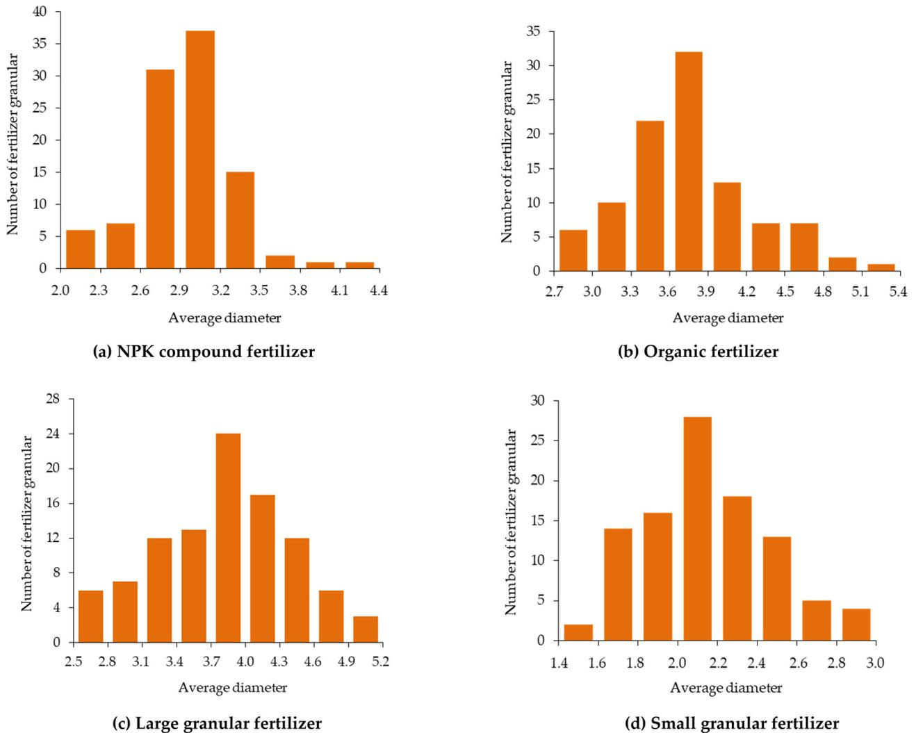
**Figure 2.** Particle size distribution of four kinds of fertilizer particles.
