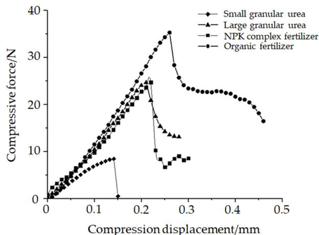
Figure 6. Compressive force-deformation curve of fertilizer granules.
