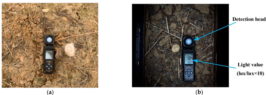
**Figure 7.** Detection of light intensity: (a) field; (b) indoor.
