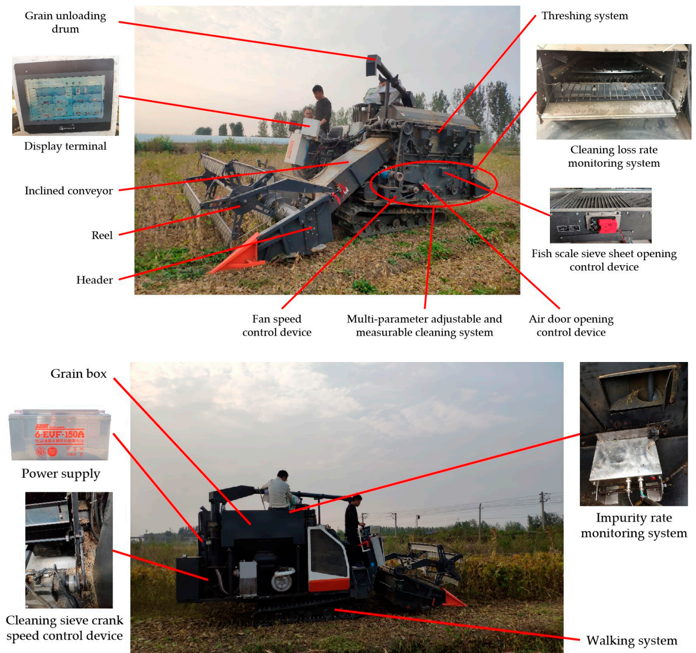
Figure 4. Prototype of adaptive cleaning system and supporting harvester.
