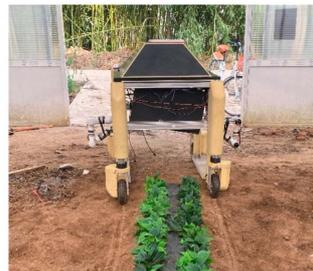
**Figure 11.** Field test environment of self-balancing mobile robot.
