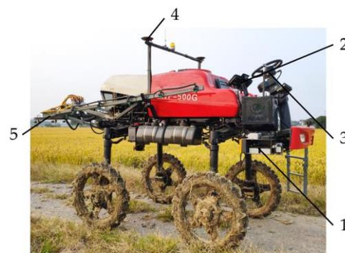
**Figure 1.** Structure of unmanned plant protection robot: 1, control system; 2, servo steering wheel; 3, human–machine interaction; 4, positioning antenna; 5, spraying valve group.
