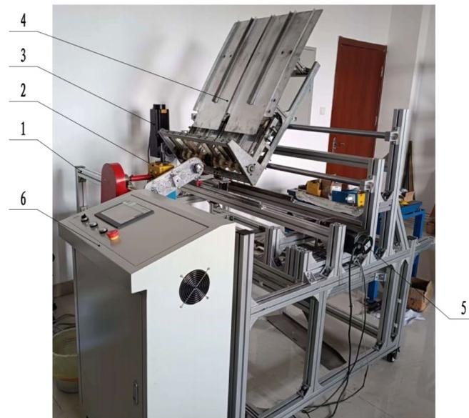
**Figure 17.** The physical picture of the transplanting mechanism test bench. 1. Frame; 2. transmission device of transplanting mechanism; 3. longitudinal seedling delivery mechanism; 4. seedling box; 5. horizontal seedling delivery mechanism; 6. control cabinet.
