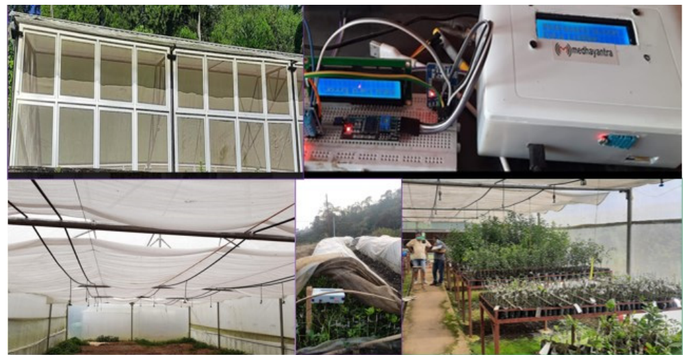
Figure 8. Implementation site: National Citrus Research Program, Dhankuta, Nepal. Figure depicts the experimental set-up for offseason grafting of Citrus fruits inside a polyhouse. The proposed IoT platform is used to regulate internal microclimate in real time.
