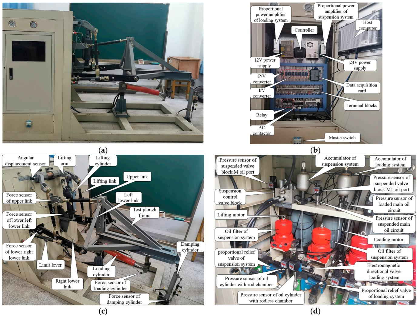
Figure 10. Test-bench physical map. (a) Integral structure; (b) Control cabinet; (c) Machine construction; (d) Hydraulic system.
