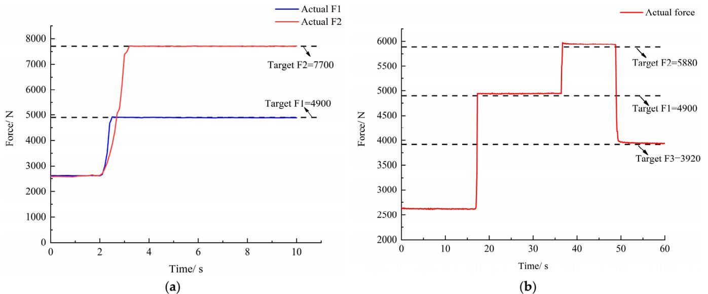
**Figure 13.** The results of loading-control test. (a) Fixed target; (b) Variable target.
