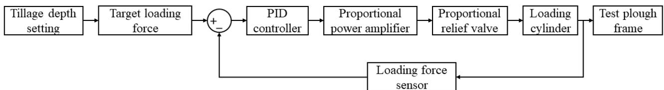
**Figure 8.** The block diagram of the loading-control system.
