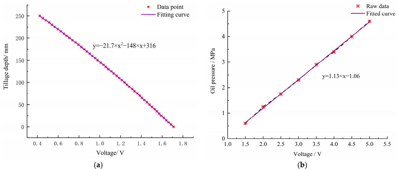
**Figure 12.** Calibration results. (a) The results of angular displacement sensor; (b) The results of electromagnetic proportional relief valve.
