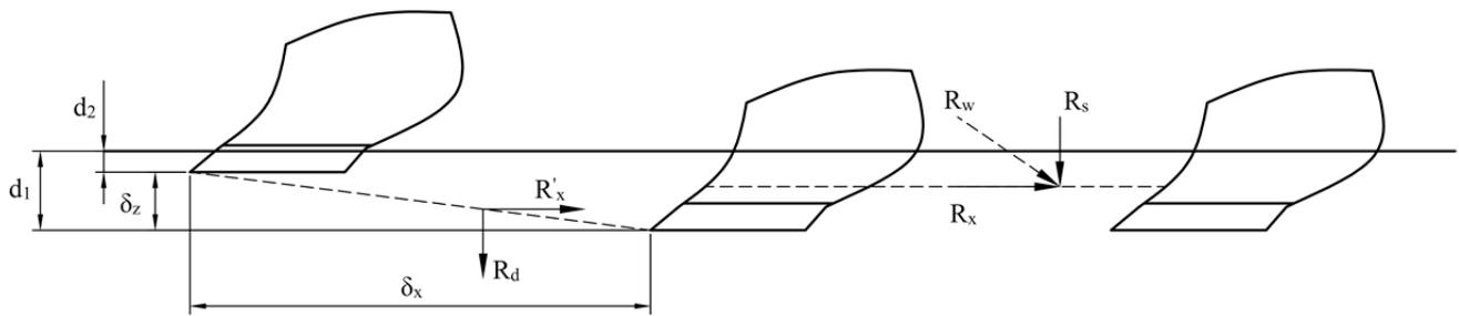
Figure 1. Force analysis of plough body.
