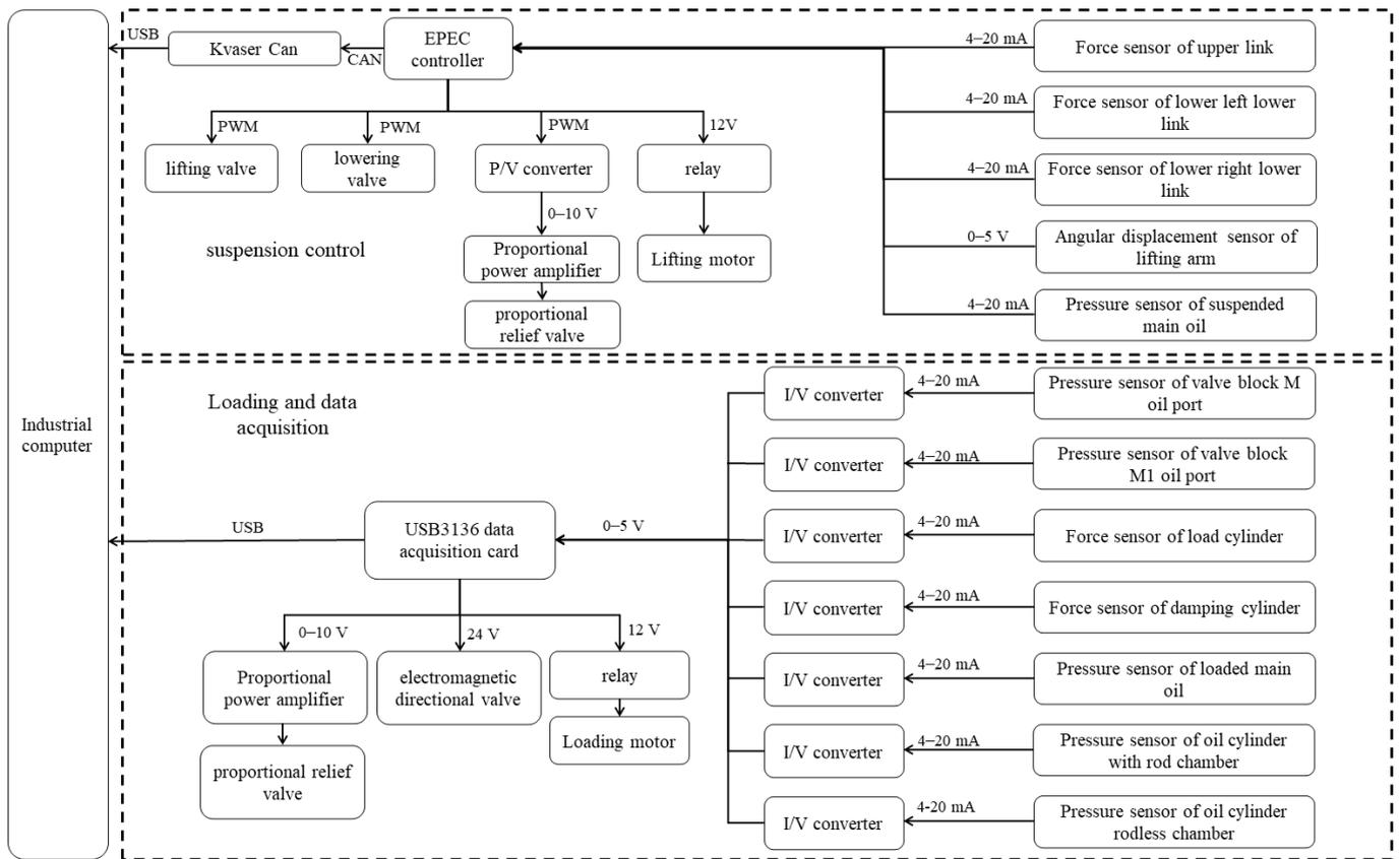
Figure 3. Hardware composition of measurement and control system.
