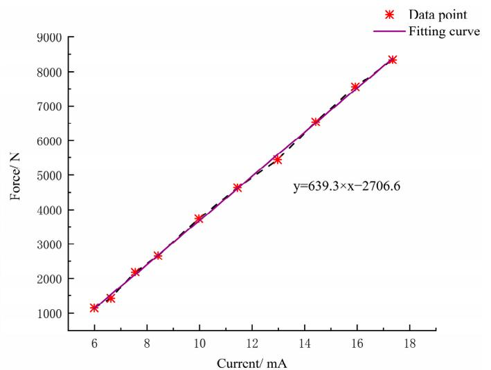
Figure 11. Calibration test of force sensor. (a) Test site; (b) Test result.
