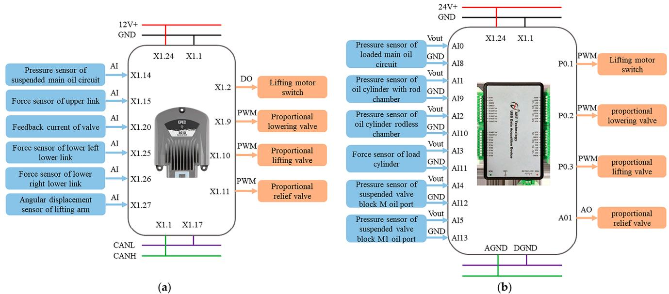
**Figure 4.** The pin definition of the EPEC3610 controller and USB3136A data-acquisition card. (a) EPEC3610 controller; (b) USB3136A data-acquisition card.
