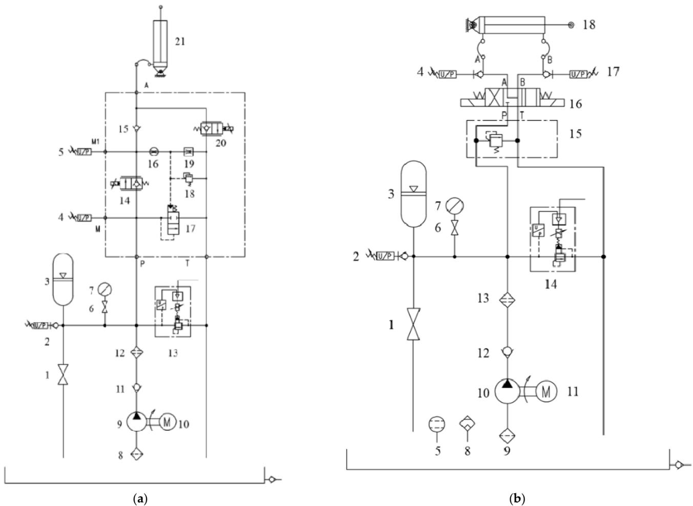
Figure 5. Hydraulic system diagram. (a) Suspension hydraulic system; (b) Loading hydraulic system. The hydraulic components represented by the serial number.
