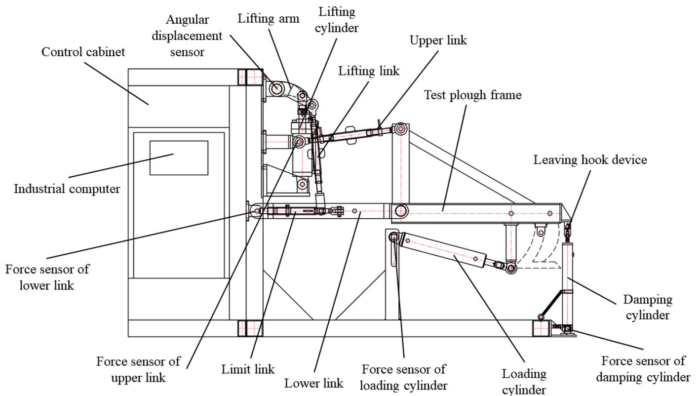
**Figure 2.** Overall structure diagram of the test bench.
