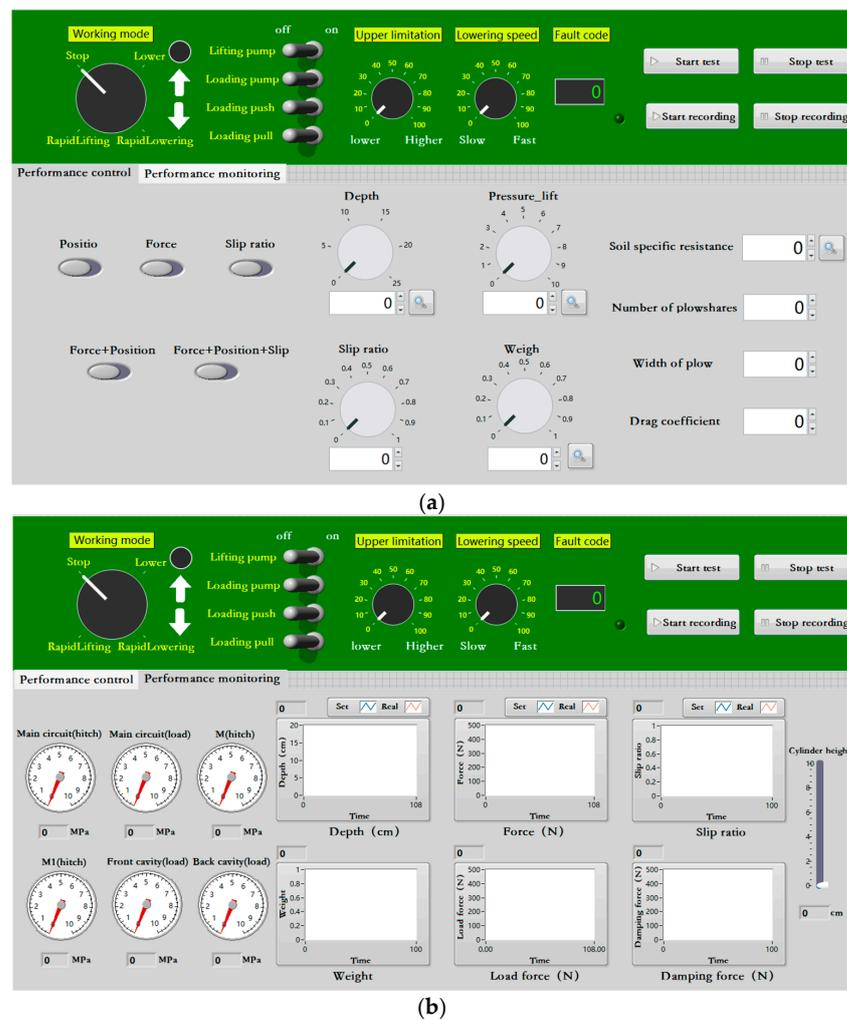
Figure 7. Measurement and control system operation panel. (a) Performance control interface; (b) Performance monitoring interface.
