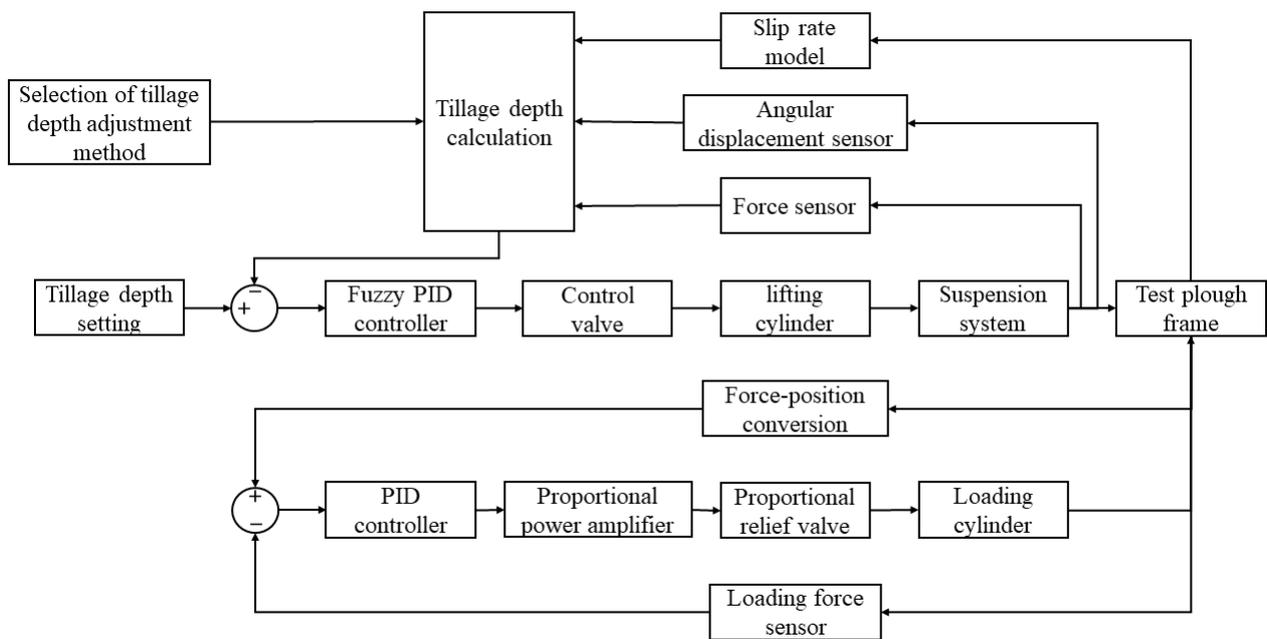
Figure 9. The block diagram of the suspension control system.
