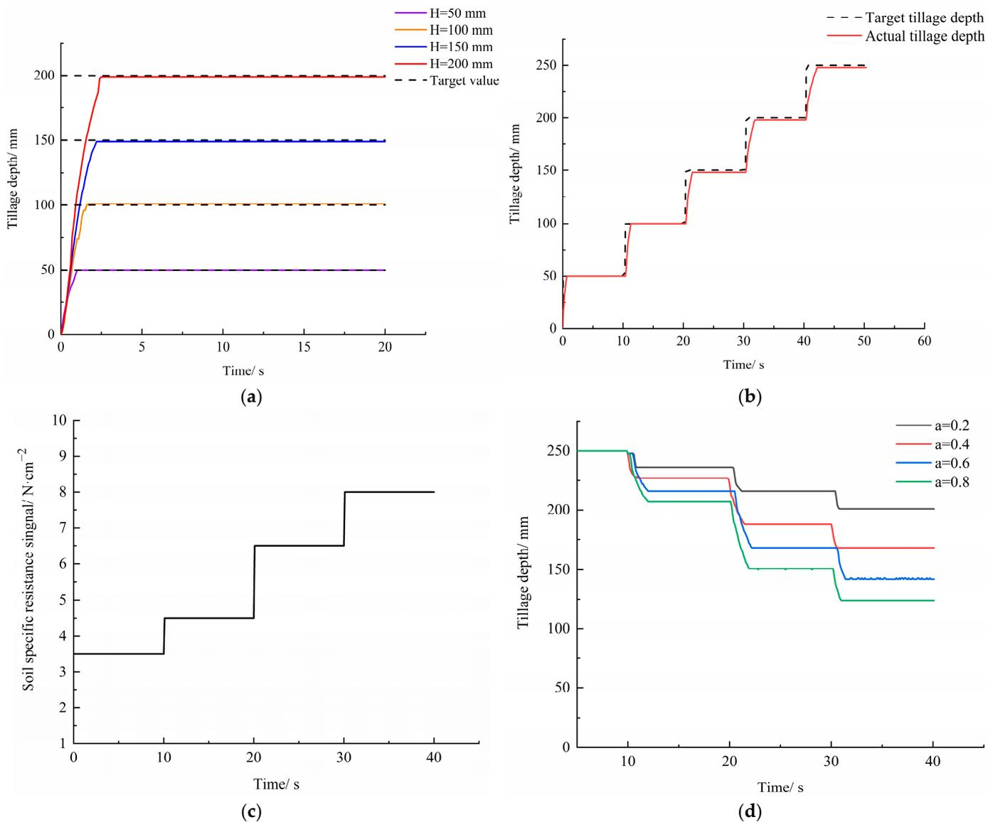
**Figure 14.** The results of tillage-depth control test. (a) Position control of fixed target; (b) Position control of variable target; (c) Soil-specific resistance; (d) Draft-position integrated control.
