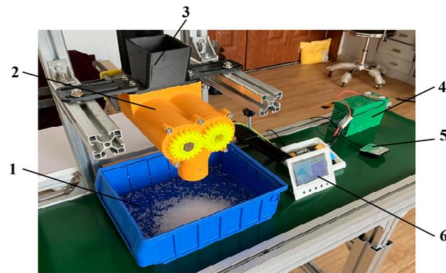
**Figure 20.** Bench test of electronic fertilizer discharge system. 1. Fertilizer collection box. 2. Optimized arc groove screw fertilizer discharge wheel. 3. Fertilizer box. 4. Motor controller. 5. GPS receiver. 6. Electronic fertilizer discharge system.
