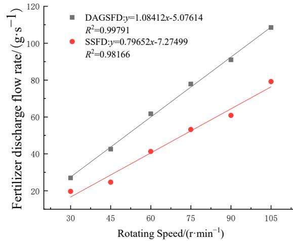
Figure 19. Fertilization discharge flow rate comparison test.
