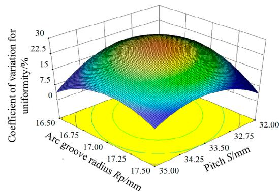
**Figure 12.** Response surface of arc groove radius and center distance to uniformity variation coefficient.
