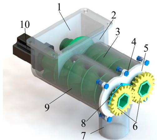
**Figure 1.** Schematic diagram of the double arc groove screw fertilizer discharger: 1. Fertilizer inlet. 2. Shell. 3. Left-handed fertilizer discharge wheel. 4. Bolt fertilizer discharge wheel. 5. End cover. 6. Gear. 7. Fertilizer outlet. 8. Direction of rotation. 9. Right-handed fertilizer discharge wheel. 10. Motor.
