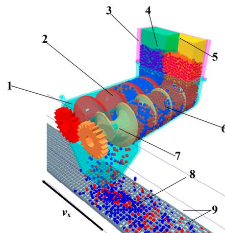
**Figure 8.** EDEM simulation: 1. Shell. 2. Left arc-groove-type fertilizer discharge wheel. 3. Fertilizer box. 4. Left fertilizer particle factory. 5. Right fertilizer particle factory. 6. Fertilizer particles. 7. Right arc-groove-type fertilizer discharge wheel. 8. Fertilizer collection tank 9. Monitoring area. Note:  $v_x$  is the movement direction of the fertilizer discharger.
