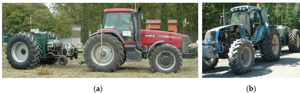
**Figure 3.** The MTB during the tests: (a) MTB on the compact surface with plant residue, pulled by a 205 kW tractor; (b) MTB and 4WD tractor with identical rear tires on asphalt track.
