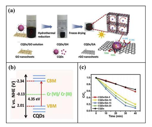
**Figure 7.** Carbon quantum dot graphene nano-aerogel: (**a**) the fabrication process; (**b**) band structure of carbon quantum dot; and (**c**) photocatalytic performance of chromium (VI) reduction during UV–Vis light irradiation. Adapted with permission from Wang et al. [106] and Lee et al. [86].
