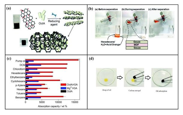
**Figure 8.** Illustration of octylamine reduced graphene oxide aerogel fabrication for oil/water separation: (a) the fabrication process; (b) organic solvent separation experiment; (c) absorption of different organic solvents and dyes; and (d) absorption performance of the aerogel. Reproduced with permission from Eom et al. [121].
