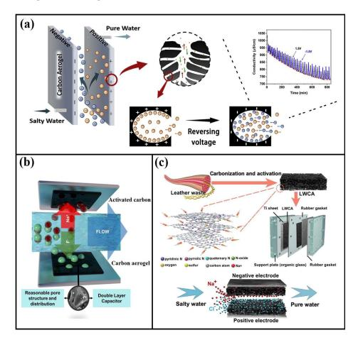
**Figure 6.** Schematic illustration of carbon aerogels for water deionization; (**a**) nanostructured carbon aerogel for capacitive deionization, adapted from Zhang et al. [99]. (**b**) Schematic diagram of carbon aerogel's electrode and its defluorination, adapted from Zhang et al. [101]. (**c**) leather waste-based carbon aerogel using one-step pyrolysis for enhanced capacitive water deionization. Adapted from Liu et al. [100].
