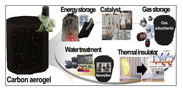
Figure 4. Illustration of carbon and activated carbon aerogel fields with applications. Adapted from [86].
