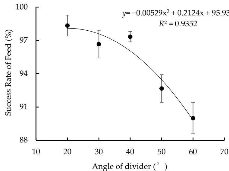
**Figure 4.** Effect of the angle of the divider on success rate of feed. Note: working speed was 1.08 km·h<sup>-1</sup>, the height of the tip of the divider's tooth from the ground was 100 mm, the ratio of the lifter's speed to working speed was 2.0 and the length of the lifter's tooth was 350 mm.
