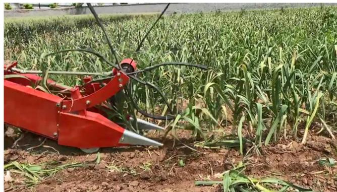
**Figure 2.** Field test of test prototype of divider and lifter mechanisms.
