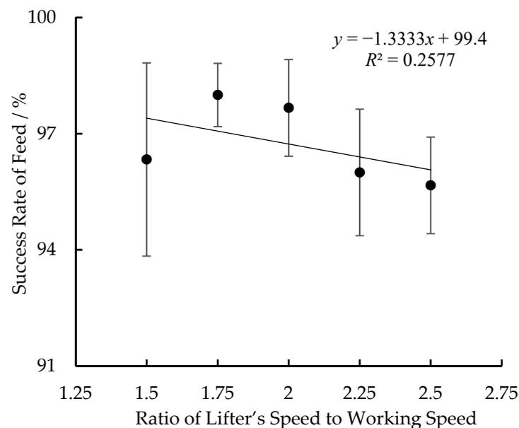
**Figure 6.** Effect of the ratio of the lifter's speed to the working speed on success rate of feed. Note: working speed was  $1.08 \text{ km}\cdot\text{h}^{-1}$ , the angle of the divider was  $40^\circ$ , the height of the tip of the divider's tooth from the ground was 100 mm and the length of the lifter's tooth was 350 mm.
