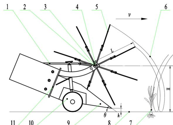
**Figure 1.** Structure of test prototype of divider and lifter mechanisms. 1. Transmission shaft; 2. gear box; 3. bearing; 4. shaft; 5. lifter's tooth; 6. trajectory curve; 7. garlic; 8. ground; 9. divider's tooth; 10. depth-limiting wheel; 11. frame.
