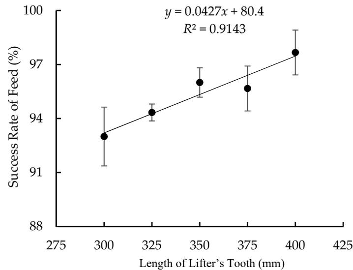
**Figure 7.** Effect of the length of the lifter's tooth on success rate of feed. Note: working speed was  $1.08 \text{ km}\cdot\text{h}^{-1}$ , the angle of the divider was  $40^\circ$ , the height of the tip of the divider's tooth from the ground was 100 mm and the ratio of the lifter's speed to working speed was 2.0.
