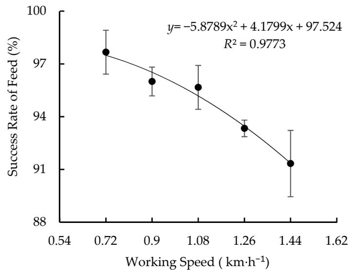
**Figure 3.** Effect of working speed on success rate of feed. Note: the angle of divider was 40°, the height of the tip of the divider's tooth from the ground was 100 mm, the ratio of the lifter's speed to working speed was 2.0 and the length of the lifter's tooth was 350 mm.
