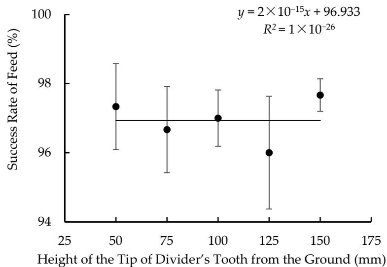
**Figure 5.** Effect of the height of the tip of the divider's tooth from the ground on success rate of feed. Note: working speed was  $1.08 \text{ km}\cdot\text{h}^{-1}$ , the angle of the divider was  $40^\circ$ , the ratio of the lifter's speed to working speed was 2.0 and the length of the lifter's tooth was 350 mm.
