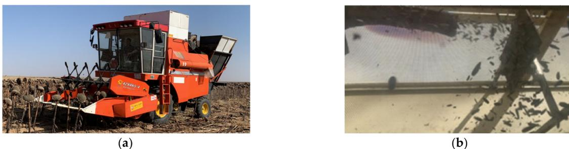
**Figure 14.** Sunflower harvesting field experiment: (a) 4ZXRKS-4 type self-propelled sunflower combine harvester; and (b) impact-type sunflower yield sensor.
