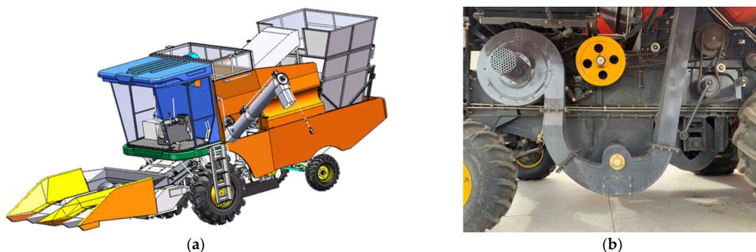
**Figure 1.** 4ZXRKS-4 type self-propelled sunflower combine harvester: (a) sunflower combine harvester structure sketch; and (b) pneumatic conveying device.
