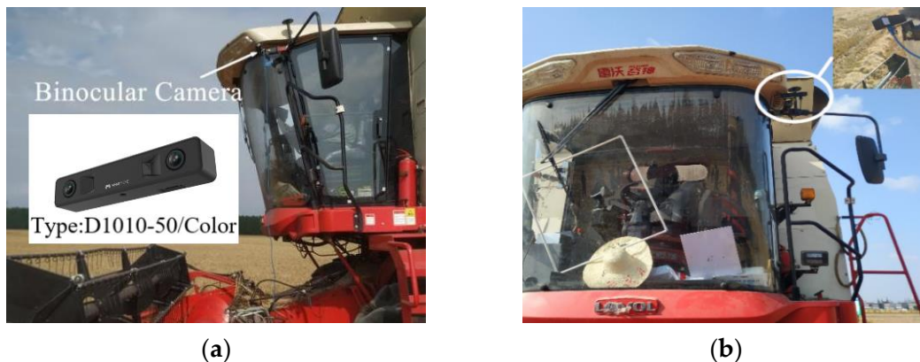
Figure 6. Binocular camera installation diagram. (a) Side view; (b) Front view.
