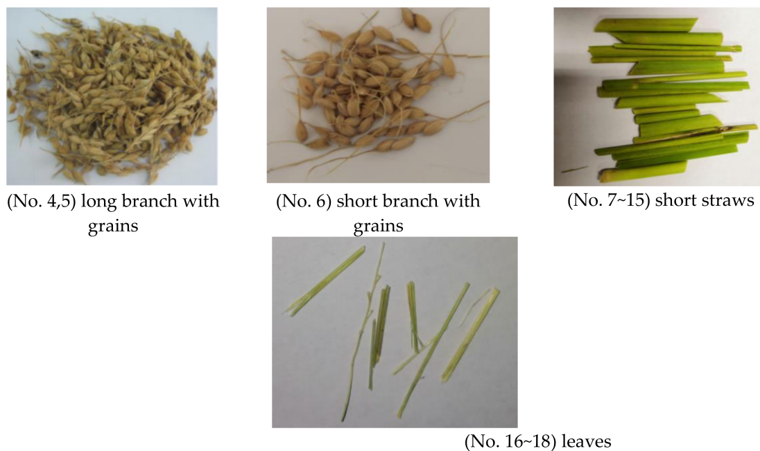
Figure 2. Illustrations of the different components in the threshing outputs for which the terminal velocity was measured.
