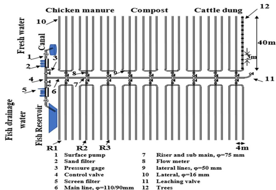
**Figure 2.** The layout of the drip irrigation system.
