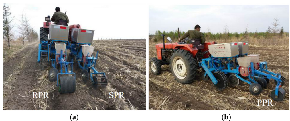
Figure 6. The types of press rollers: (a) the RPR and SPR; (b) the PPR and SPR.
