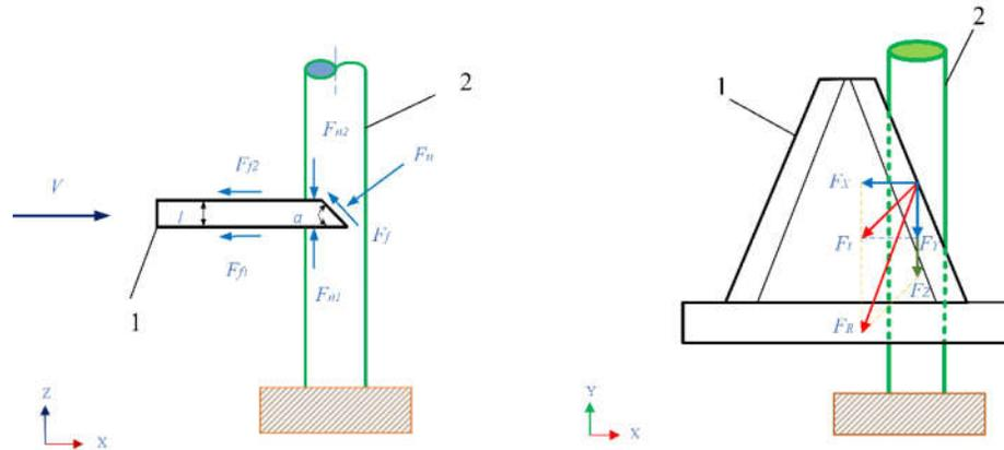
**Figure 2.** Cutting force analysis of cutting blade stem.
