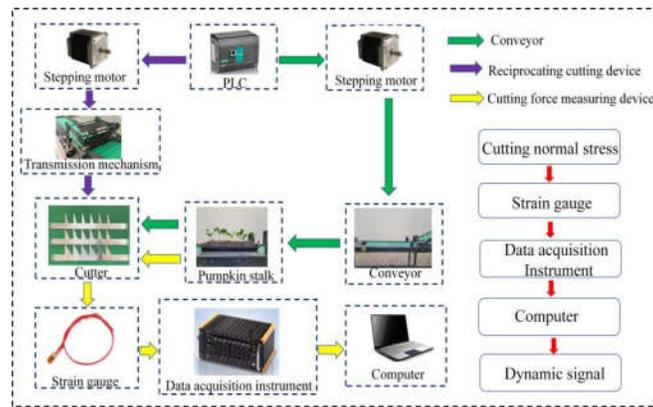
**Figure 13.** Structure diagram of high-speed grafting experiment bench for vegetable grafted seedlings.
