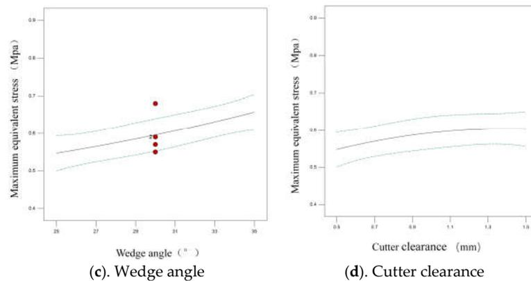
**Figure 8.** The influence of each single factor on the maximum cutting stress.
