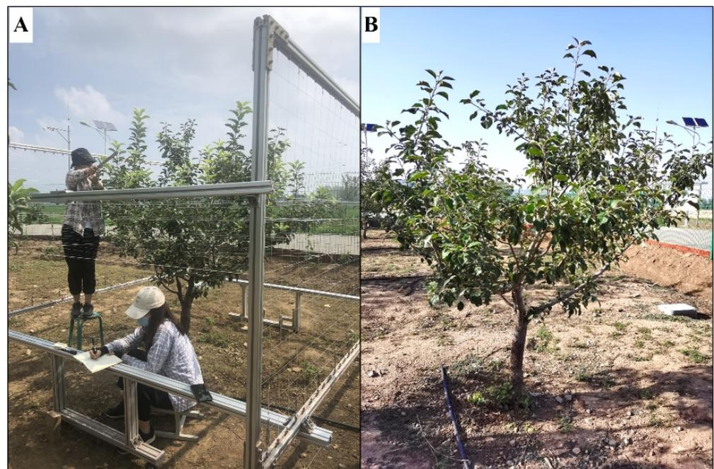
**Figure 1.** Manual measurement process of canopy leaf area (A) and the test orchard tree (B).
