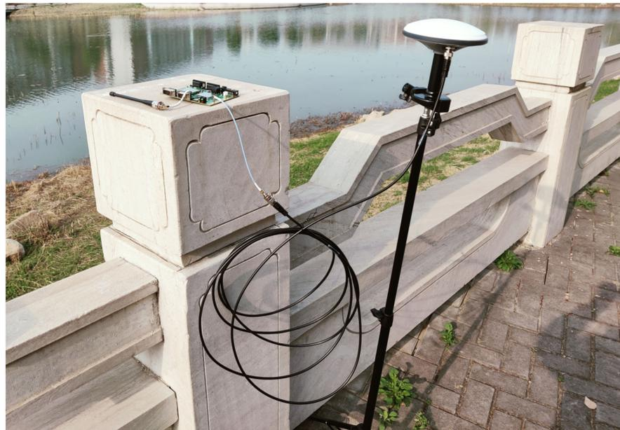
**Figure 5.** Differential reference station.
