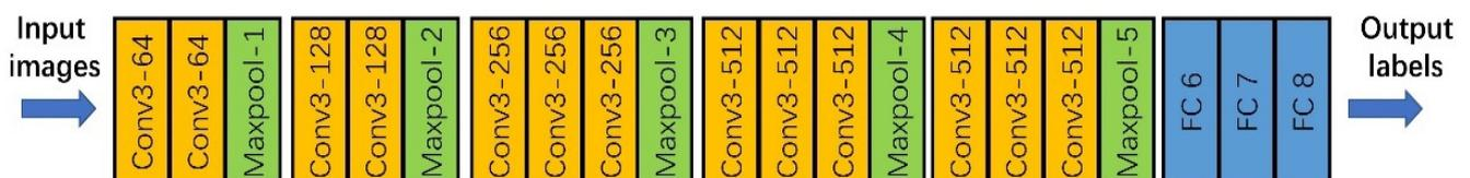
**Figure 7.** Structure diagram of VGG-16.
