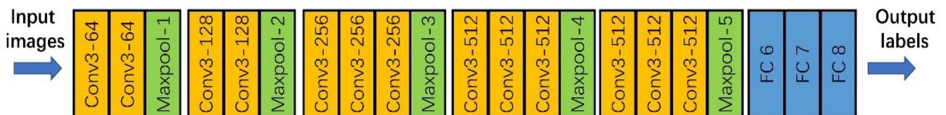
Figure 7. Structure diagram of VGG-16.
