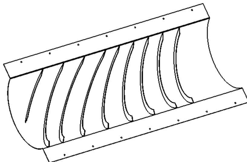
Figure 6. Threshing room upper cover structure.
