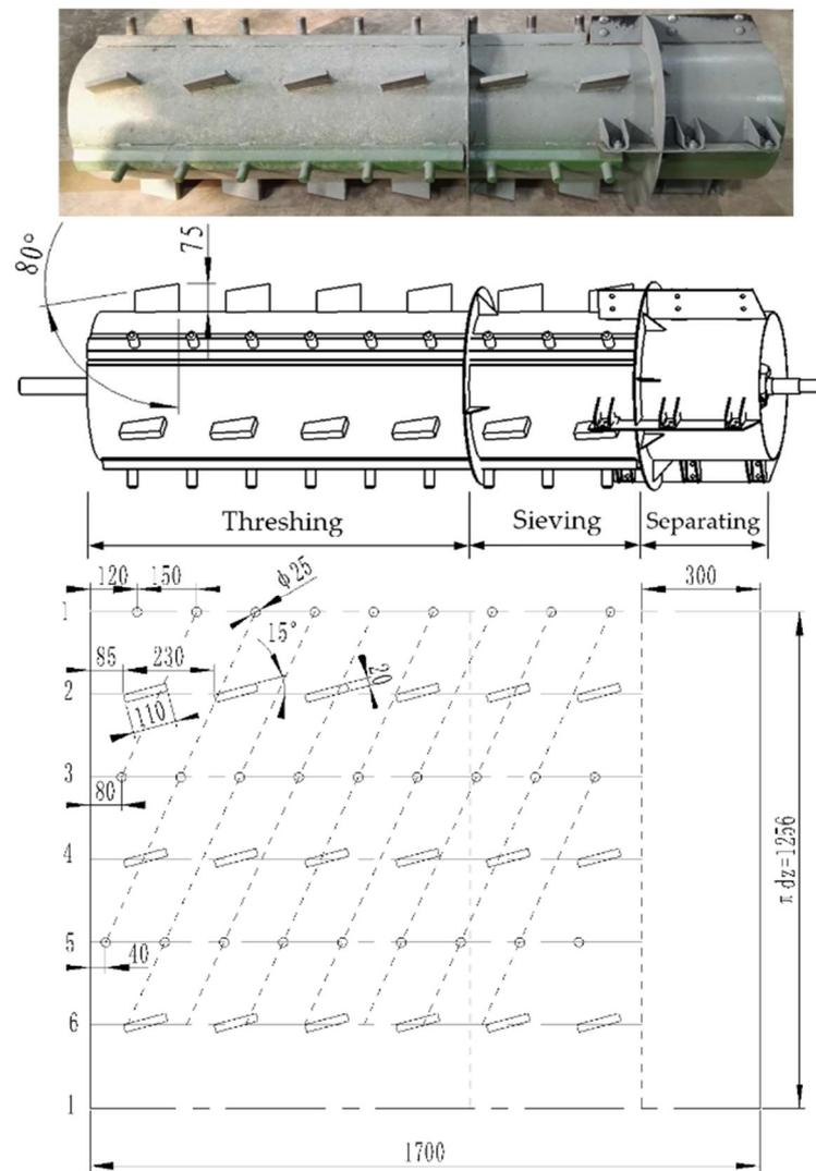
**Figure 3.** Transverse axial flow drum structure and the column tooth-plate's tooth arrangement (magnified view).
