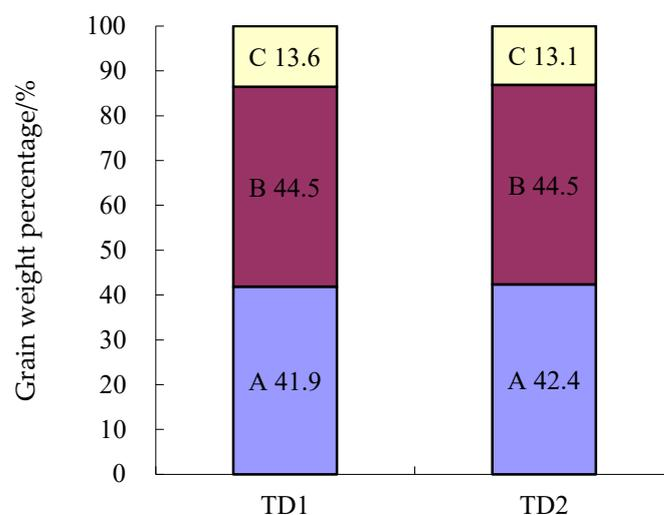
**Figure 8.** Threshing amount statistical comparison in different sections of two types of drums.
