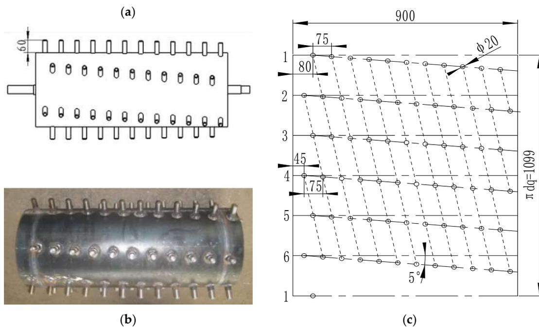
**Figure 2.** Tangential flow drum structure and column tooth arranged expanded view (magnified view). (a) The 3D model, (b) physical picture, (c) column teeth arranged expanded view.
