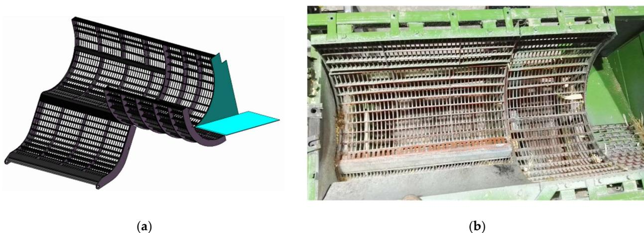
**Figure 5.** Concave plate sieve assembly. (a) The 3D model; (b) physical picture.
