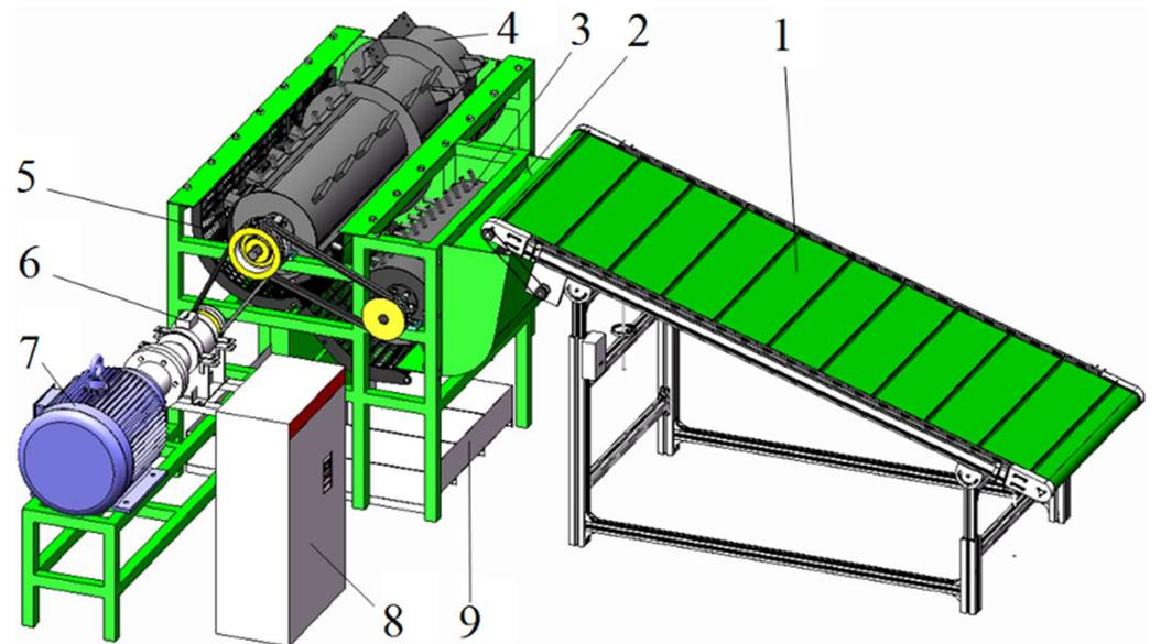
**Figure 1.** The 3D maize threshing test bench. (1) Feeding device; (2) feeding port; (3) tangential flow drum; (4) axial flow drum; (5) grid grating; (6) torque speed sensor; (7) motor; (8) electrical control cabinet; (9) grain collection box.
