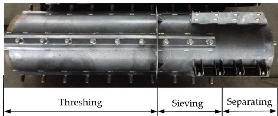
**Figure 4.** The fullcolumn tooth threshing drum (TD2 for short).
