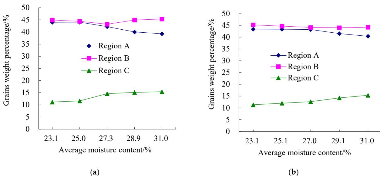
**Figure 9.** The relationship between threshing grain amount and moisture content in each section. (a) TD1; (b) TD2.
