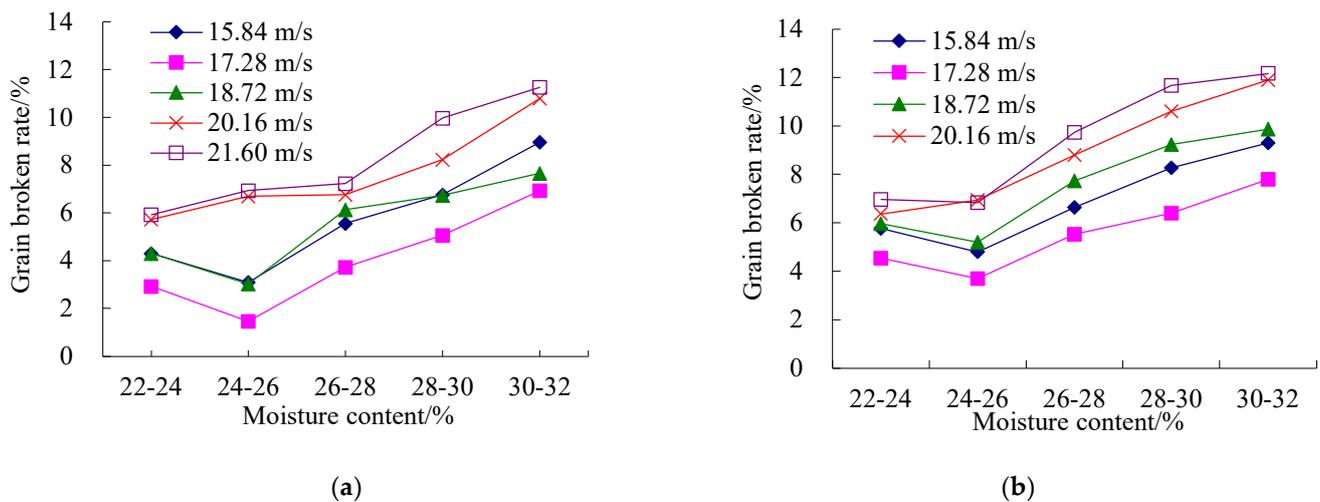
**Figure 12.** The relationship between the moisture content and grain broken rate under various drum peripheral velocity conditions. (a) TD1; (b) TD2.
