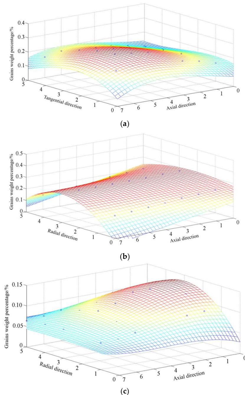
**Figure 11.** Threshing flow distribution variation law quadratic response surface. (a) Tangential flow threshing zone A; (b) transverse axial flow threshing zone B; (c) transverse axial flow threshing zone C.
