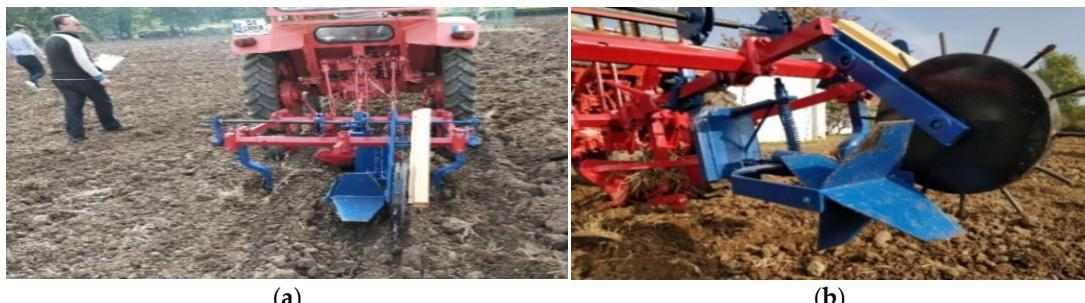
**Figure 15.** Testing the furrow diking system equipped with the standard rotor blades. (a) Testing the equipment performance on difficult soils. (b) Evaluation of the equipment wear during testing.
