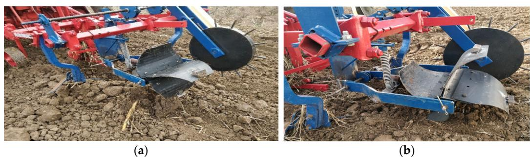
**Figure 18.** Testing the furrow diking system equipped with the curved rotor blades. (a) Testing the equipment performance on difficult soils. (b) Evaluation of the equipment wear during testing.
