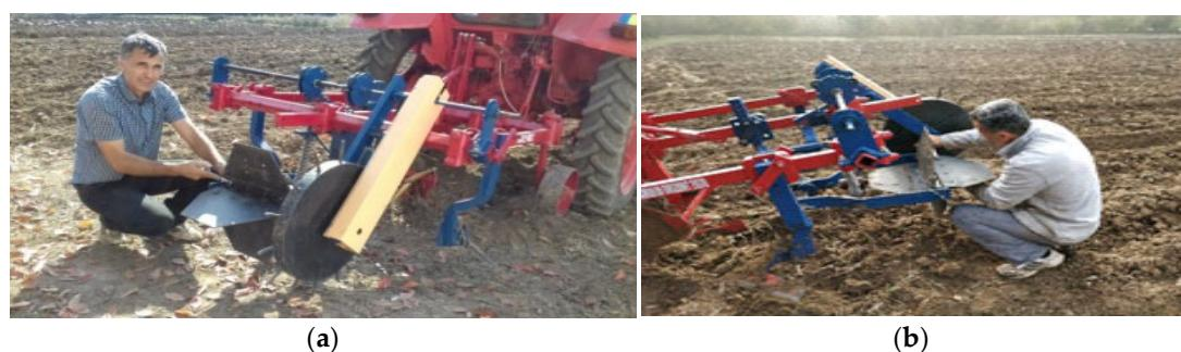
**Figure 16.** Testing the furrow diking system equipped with the optimized straight rotor blades. (a) Testing the equipment performance on difficult soils. (b) Evaluation of the equipment wear during testing.
