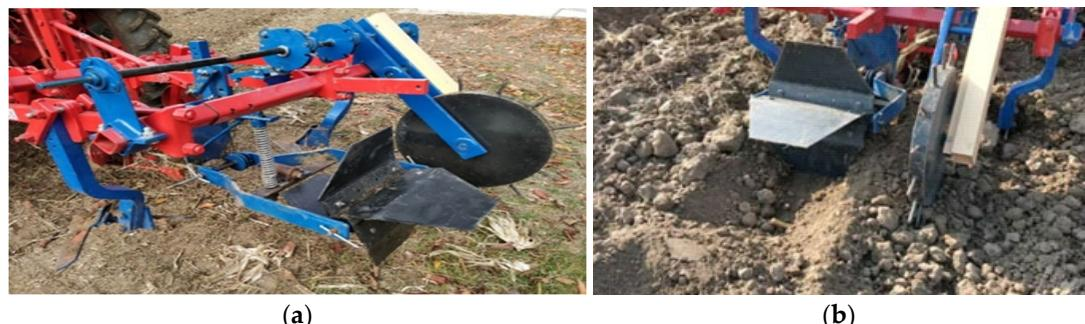
**Figure 17.** Testing the furrow diking system equipped with the inclined rotor blades. (a) Testing the equipment performance on difficult soils. (b) Evaluation of the equipment wear during testing.
