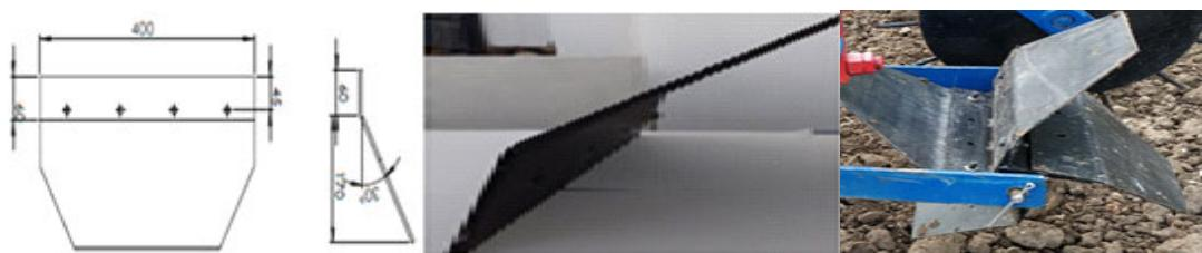
**Figure 9.** Design and construction of an inclined optimized blade equipped with the furrow compartmenting system rotor.
