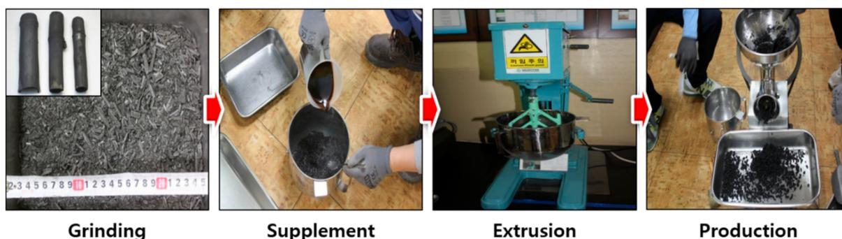
**Figure 1.** Manufacturing process of pelleted biochar (BC\_PT) using bamboo biochar.
