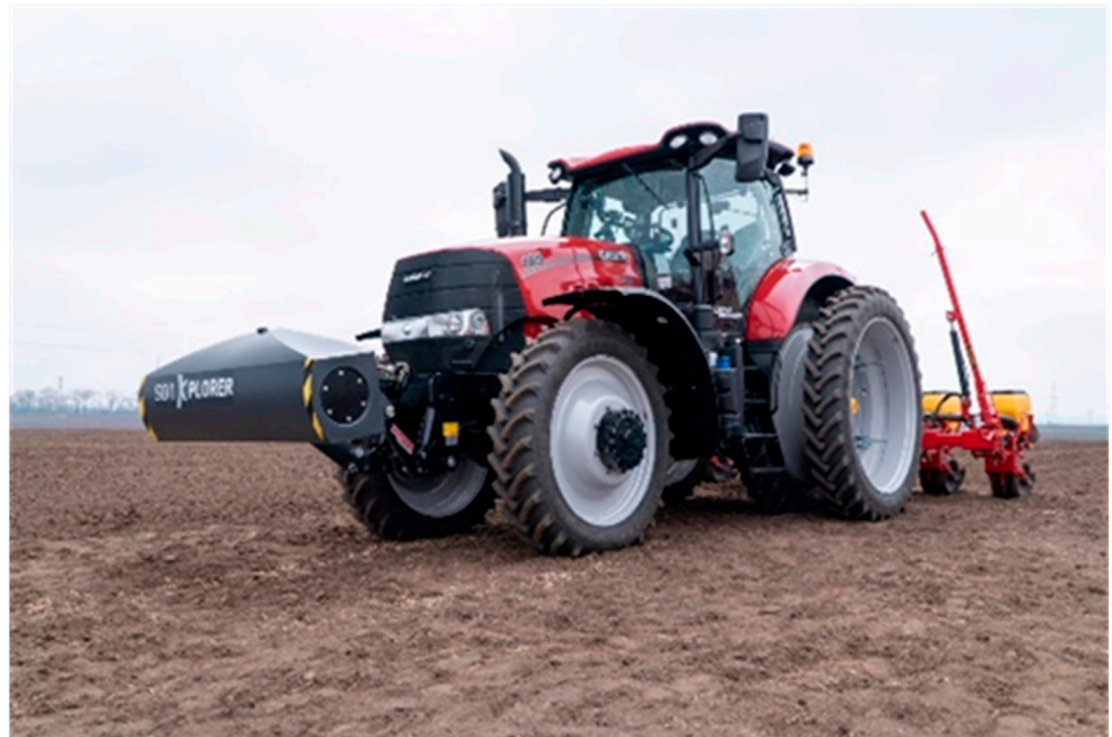
Figure 12. SoilXplorer device for measuring soil structure differences [60].
