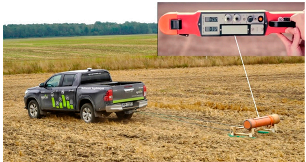
Figure 9. EM38-MK2 remote sensing device constructed on a plastic sledge [22].
