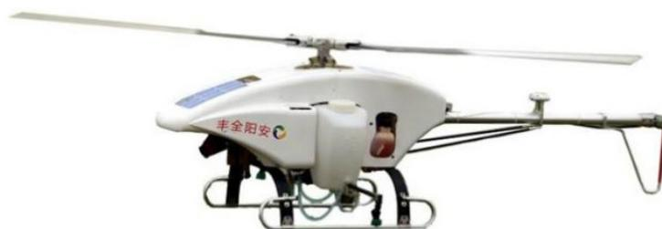
**Figure 1.** 3WQF120-12 plant protection UAV.
