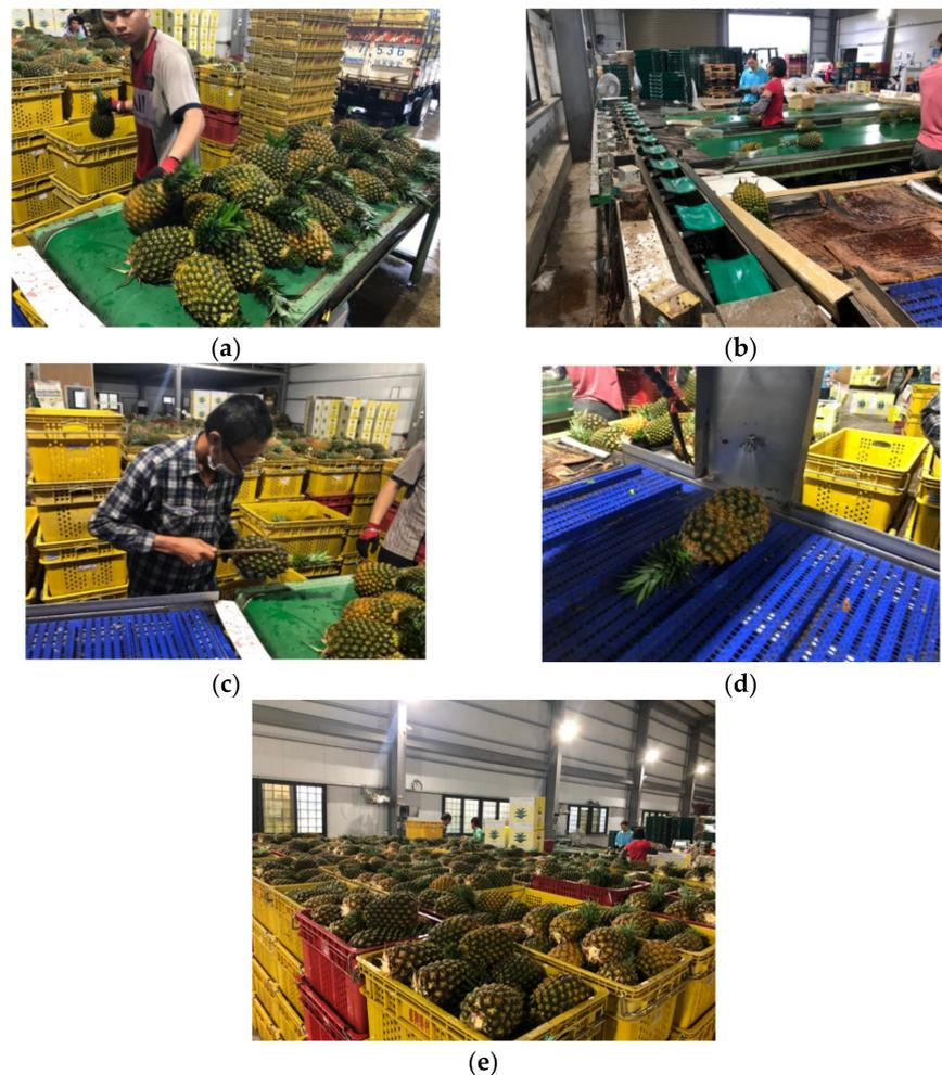
**Figure 1.** Time and resource-consuming classification of pineapples; (a) transportation, (b) conveyor classification by weight, (c) sound test classification, (d) cleaning, and (e) final classified pineapples.
