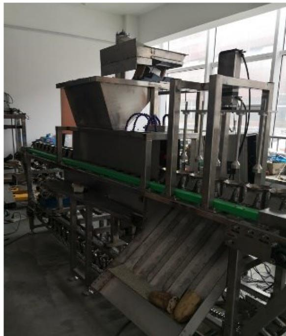
**Figure 5.** Prototype of automatic rice-filling device for lotus root with glutinous rice.
