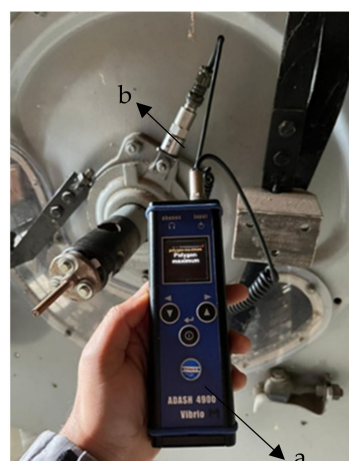
Figure 5. a. Adash A4900 Vibrio M device; and b. AC150 piezoelectric sensor.
