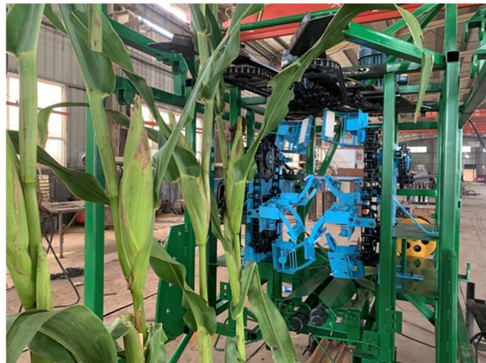
**Figure 8.** Ear picking test bench for fresh corn.
