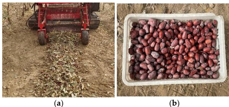
**Figure 15.** (a) Field test of a floor-standing jujube pickup device. (b) Jujubes picked up by devices.
