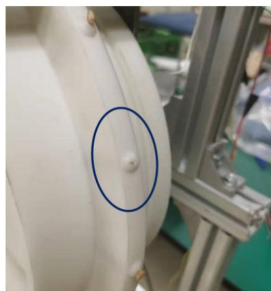
Figure 26. Seed leakage.
