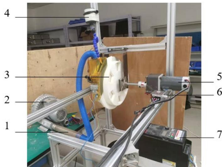
**Figure 24.** Experiment bench. Note: 1, Air suction pipe; 2, Experiment fan; 3, Sees drill; 4, Air blower; 5, DC motor; 6, DC motor controller; 7, Fan controller.
