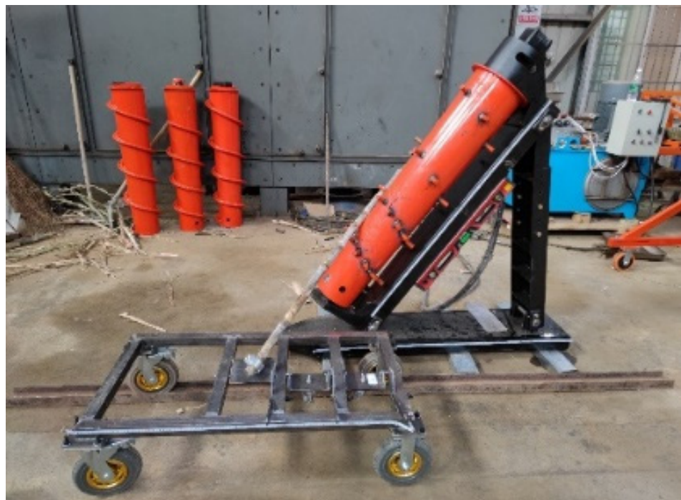
Figure 9. Test bed for spike-toothed crop divider.
