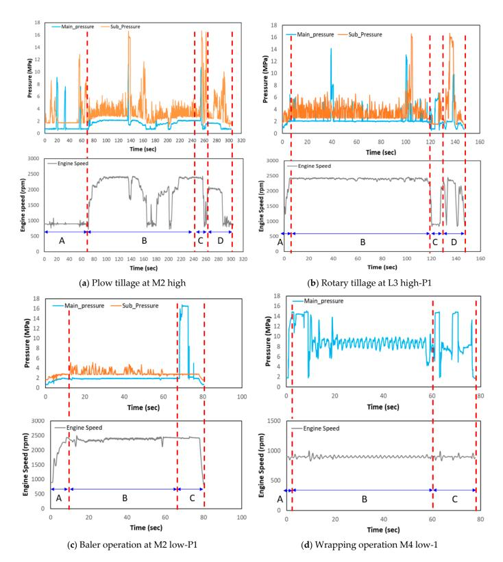
Figure 3. The pressure and engine rotational speed for major agricultural operations.
