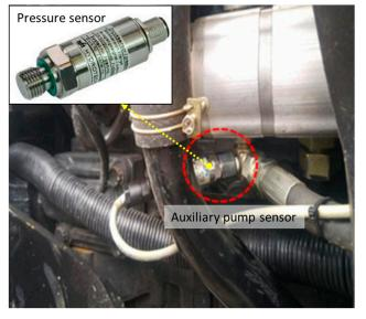
(b) Auxiliary pump pressure sensor
