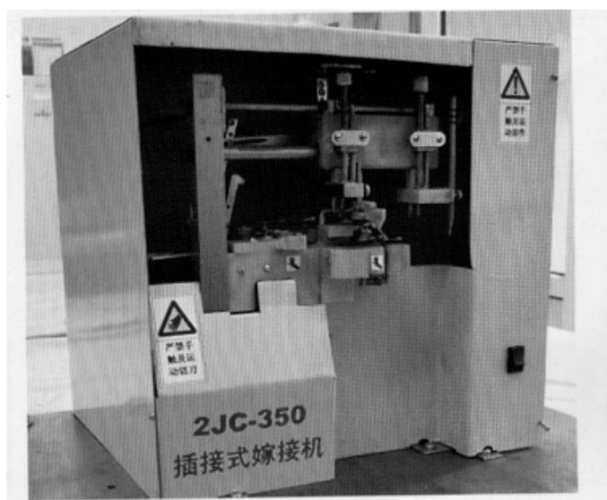
**Figure 6.** 2JC-350 plug-in semi-automatic grafting robot developed by Northeast Agricultural University.
