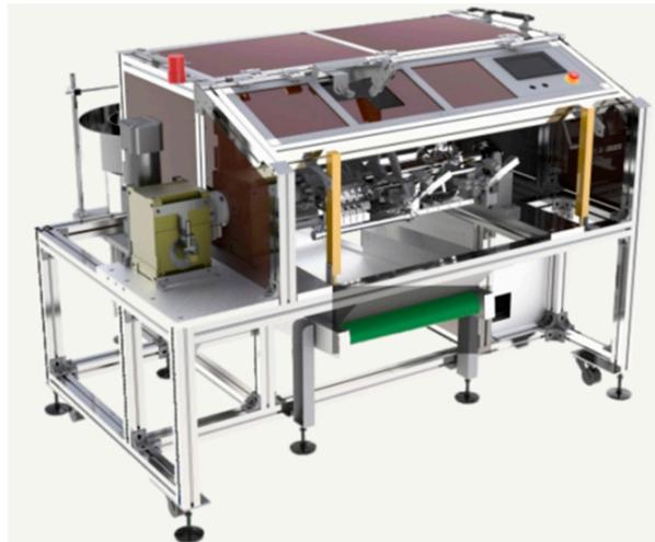
**Figure 2.** JFT-A1500T semi-automatic grafting robot developed by Hefei Jiafute Robot Technology Co., Ltd.
