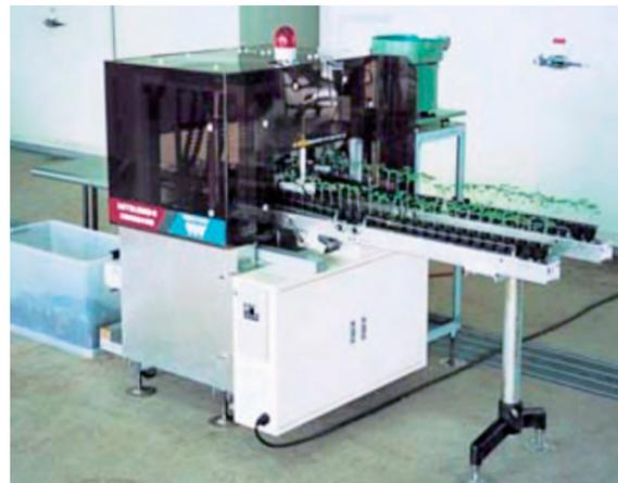
**Figure 4.** MGM600 semi-automatic grafting robot developed by Mitsubishi Group.
