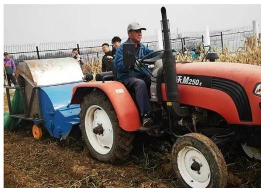
**Figure 9.** Test on double-roller sweet potato vine crushing and collecting.
