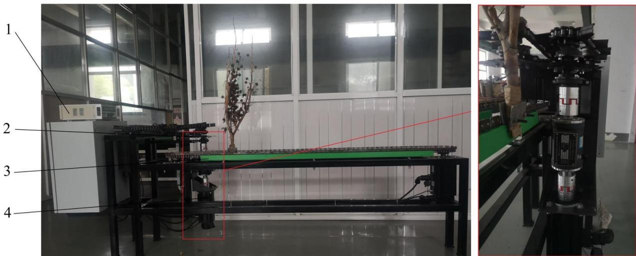
**Figure 4.** Castor disc-cutting device. (1) Measuring and controlling system. (2) Cutting system. (3) Feeding system. (4) Power system.
