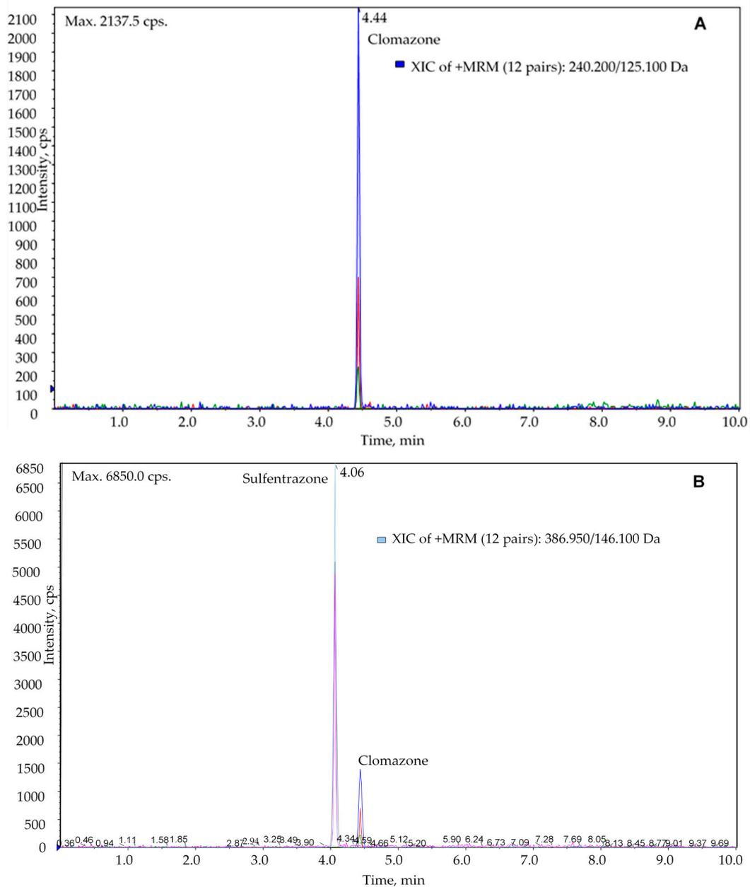
**Figure 1.** Chromatogram of sample of solutions that percolated the sugarcane straw. Application of clomazone formulations (A); application of clomazone formulations combined with sulfentrazone (B).
