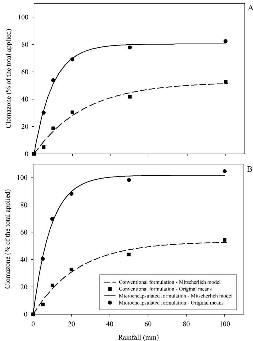
**Figure 2.** Quantity of clomazone (% of the total applied) percolated through sugarcane straw as a function of different simulated rainfall depths (mm), after application of different formulations. Application of clomazone formulations (A); application of clomazone formulations combined with sulfentrazone (B).
