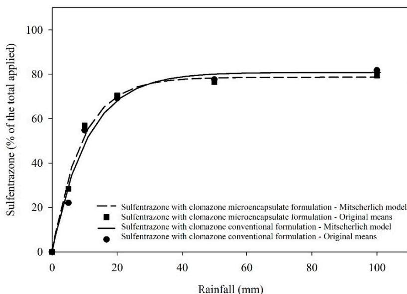
**Figure 4.** Quantity of sulfentrazone herbicide (% of the total applied) percolated through sugarcane straw as a function of different simulated rainfall depths (mm), after application combined with emulsifiable concentrate formulation (EC) or microencapsulated formulation (CS) of clomazone.
