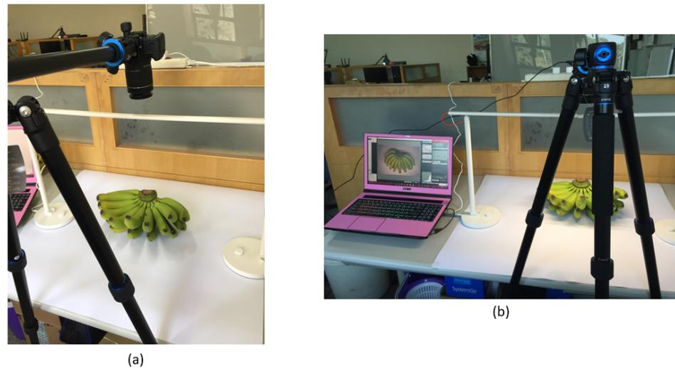
**Figure 1.** Experimental setup for obtaining RGB images of bananas, (a) white background with constant camera height, and (b) capture and image resizing software.
