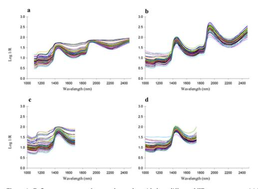
**Figure 3.** Reflectance spectra of scanned samples with four different NIR spectrometers: (a) Dispersive benchtop instrument (NIRSystem 5000); (b) FT-NIR benchtop instrument (NIRFlex N-500); (c) Diode array portable instrument (Corona 45); (d) MEMS portable instrument (LAB POD<sup>TM</sup>) reproduced from [71], with permission from ELSEVIER, 2021.
