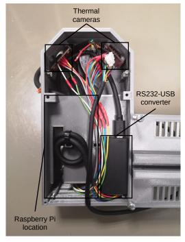
(c) Bottom-view of the hardware module showing the interior area of its case with the two thermal cameras, the Raspberry Pi location and the RS232-USB adapter.
