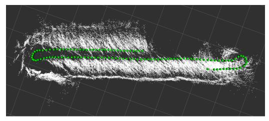
Figure 10. Laser scanning-based 3D point cloud with the path travelled by the tractor in green dots.
