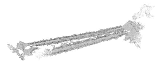
Figure 11. Resulting octree of the conversion from point cloud data.
