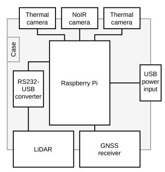
Figure 2. High-level scheme of the hardware module showing the connections between its components.
