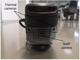
(**b**) Front-view image of the hardware module showing the two thermal cameras and the NoIR camera.
