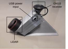
(a) Side-view image of the module showing the LiDAR, the GNSS receiver and the USB power input.
