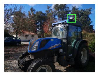
Figure 3. Tractor with the hardware module mounted on top (inside the green rectangle).
