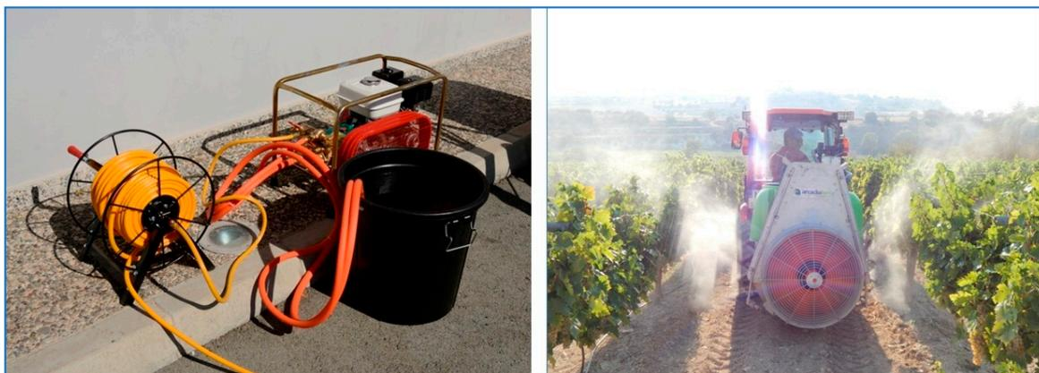
**Figure 3.** Sprayers tested. On the left the high-volume sprayer (HVS) with the spray gun and on the right the orchard sprayer (OS) used for the OS500 and OS250 treatments.
