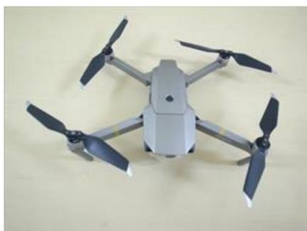
**Figure 1.** The quadrotor drone (Mavic Pro Platinum) used in the study.
