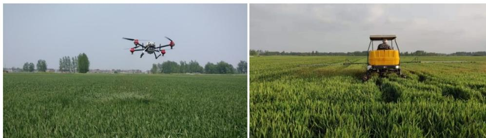
**Figure 1.** The UAV sprayer and tractor-mounted boom sprayer.
