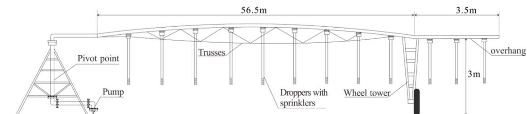
**Figure 3.** Main units and parameters of the center pivot irrigation system (CPIS).
